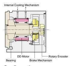
There is no mechanical reduction mechanism such as worm system in a rotary table with DD motor. DD (Direct Drive) motor is built in the the rotary table to drive directly. High rotation speed and high acceleration/deceleration can be done. However, the driving torque of the rotary table is not strong due to no mechanical reduction mechanism. Therefore, the suitable application of the rotary table with DD motor must be selected.
