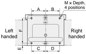
Please refer to the above dimensions for direct mounting with the bolts from base plane side.
