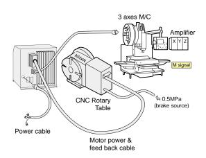
■ EZ controller (2 units) connection for 5AX tilting rotary table (2-axis)
