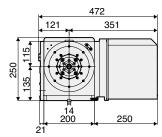
External dimensions depend on the type of the servo motor. Indicated dimensions are in case of FANUC. Please contact us for CAD files (2D:DXF, 3D:PARASOLID).
