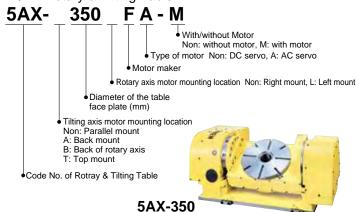
Multi-Spindle CNC Rotary Table
