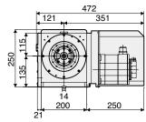
External dimensions depend on the type of the servo motor. Indicated dimensions are in case of FANUC. Please contact us for CAD files (2D:DXF, 3D:PARASOLID).
