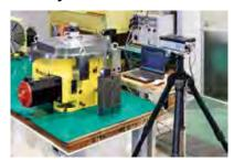
**Indexing Accuracy Measurement** by Laser
