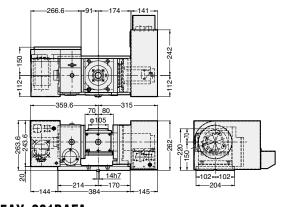
5AX-201BAFA The tilting axis motor is mounted at back side.
