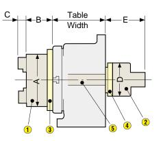
When power chuck or rotary cylinder is installed on 5AX-table, the 5AX-table must be High Column type.
