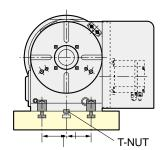
CLAMPING DEVICE is designed for T-slot pitches of 100mm or 125mm on the machine bed table. Please contact with us for the other pitches.
