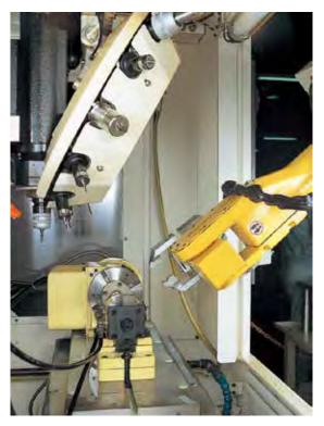
AWC magazine, Disc type, Chain type, Horizontal type and Bar Work type are available.
