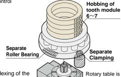
CNC1201 Indexing of the turbine shaft. Turbine shaft is supported and clamped by the roller support.
