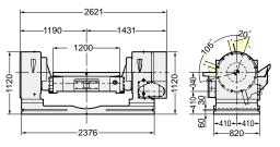
Motor capacity of rotary axis and tilting axis are added at the end of Code No. e.g 5AX-1200WA21-4444
