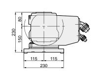
■ The Area of Noninterference in Tilting Position.
