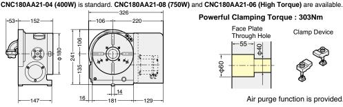
Powerful Clamping Torque: 303Nm
