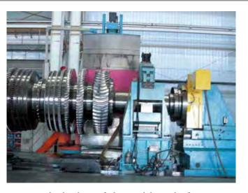
Indexing of the turbine shaft
