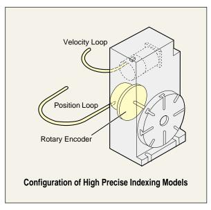
Full closed loop control becomes possible by mounting a rotary encoder at the back of rotary table. And high precise indexing becomes possible by detecting the rotary angle of the table directly.
