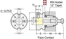
Standard Pull Stud: PS-3 Holder with ID, Pull Stud with ID are available. (optional)
